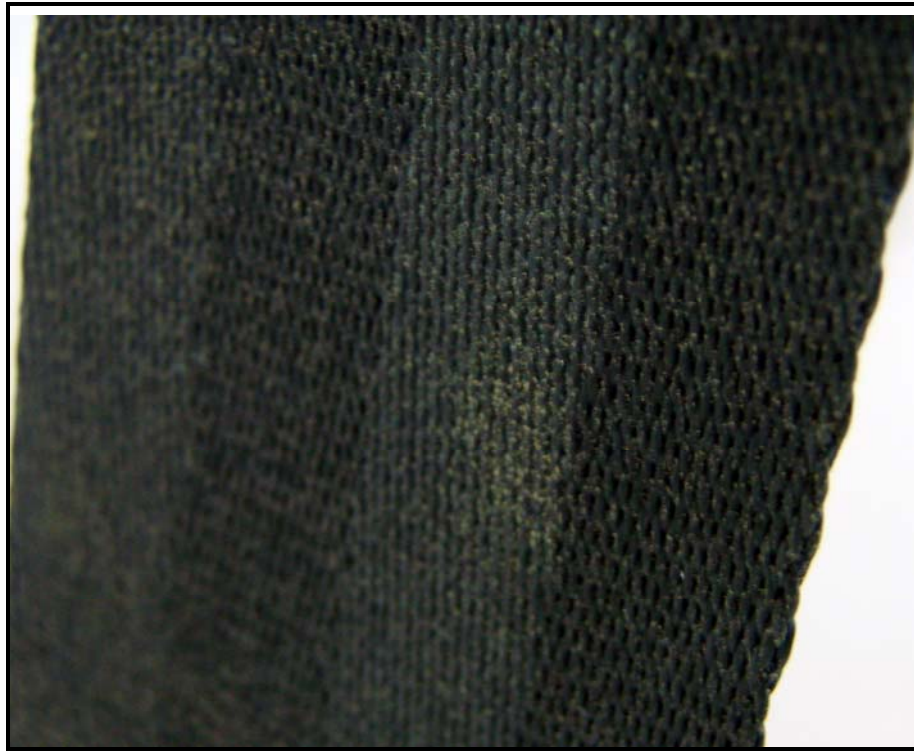
The trace amount of fungal growth was found all over the fabric part of the sample, the growth was short, thin and scattered all over the tested surface.
