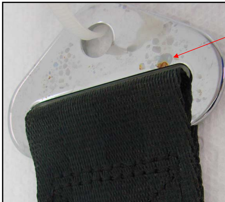
This metal piece from sample: Belt, Buckle; 682-42-13-01-1-1; Lot: 51002600 had slight discoloration/rusting present after 28 days incubation.
